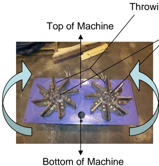
If the blast wheels were removed, place the wheel hubs back on the motor shafts and bolt on the impellers with a 3/8" Allen wrench.
