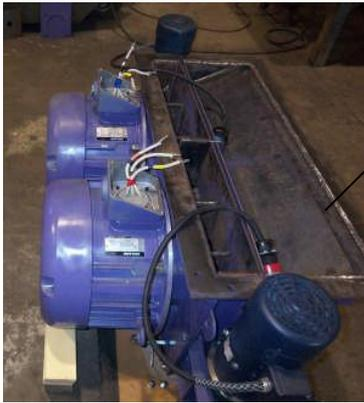
Tip the unit upright and place a block under the blast motor
