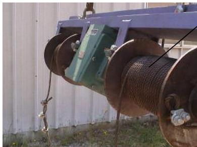
Make sure that the cable wraps on the hoist drums are straight and smooth across the drum.
