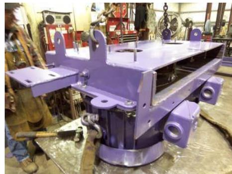
Use a fork lift to place the unit in the tank. Place the forks together on the ground under the unit, and slide the two motors onto the forks. After the unit is inside the tank, lift the unit off of the forks and onto the floor. Two men on each side can lift the unit.
