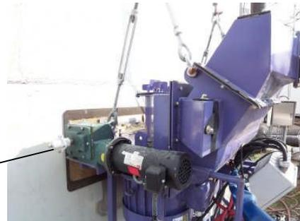
Check to make sure that the machine is hanging square to the wall. Adjust the turnbuckles if required.
