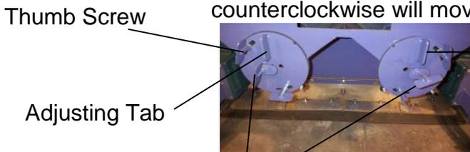
To adjust the blast pattern, loosen the thumb screws and tap the adjusting tab with a hammer to rotate the control cage. The optimum position is usually with the thumb screw stud centered in the slot as shown.
