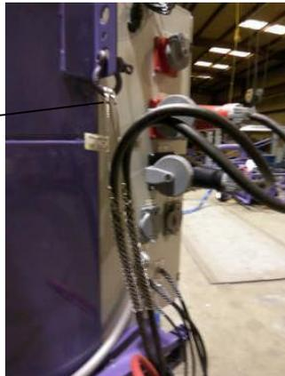
Plug in the blast machine wiring harness. Connect the cable support sling to a shackle on the dust collector. This keeps slack between the sling and the plugs so wires are not pulled loose when moving the dust collector.
