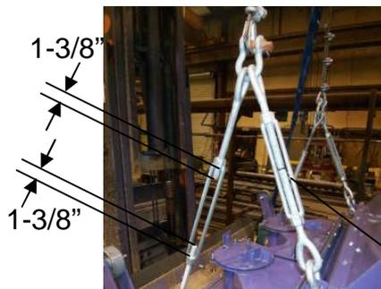
Connect the short  $\frac{3}{4}$ "x9" turnbuckle on the lifting lug located on the Hood Assy. Use a  $\frac{5}{8}$ " shackle.
