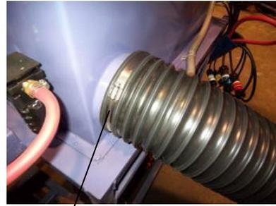
Connect 75' of standard exhaust hose to the dust collector. Leave the clamp loose for now; the hose will have to be adjusted to remove twists and loops after the fan is started.
