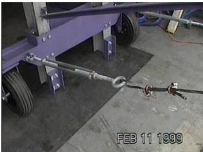
Run the cable from the turnbuckle through the rear eye and around the tanks center stand pipe. Run the cable back through the other rear eye and connect it to the opposite turnbuckle, using at least two 3/8" cable clamps. Pull the cable tight as possible before clamping. Next, pull the two cables together and place a single clamp about two foot from the stand pipe. This will keep the fixture running square to the tank.
