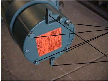
5. Slip the brake assembly off of the motor shaft being careful not to pull on the brake electrical wires. Support the brake to prevent stress on the wires while cleaning the brake.
