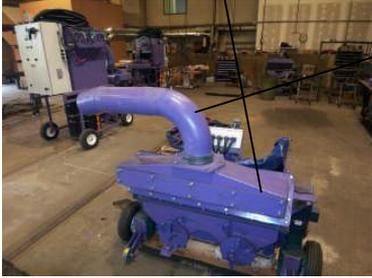
Replace the exhaust elbow
