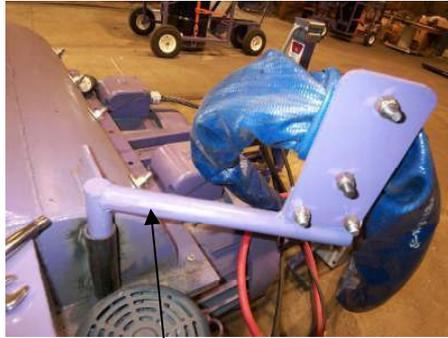
Remove the cable harness support by lifting it out of the support tube.
