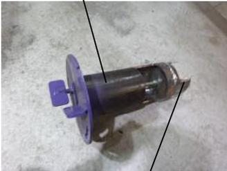
Remove the Control Cages and inspect the wear on the hard faced areas of the two Control Cages.
