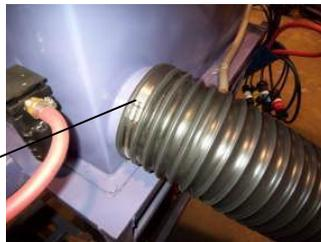
With the fan running, rotate all twists and loops out of the exhaust hose. The hose must be straight to minimize damage and pressure drop. If the suction of the dust collector is too great to rotate the hose, turn Off the fan and rotate the hose as the fan slows down. Tighten the hose clamp.
