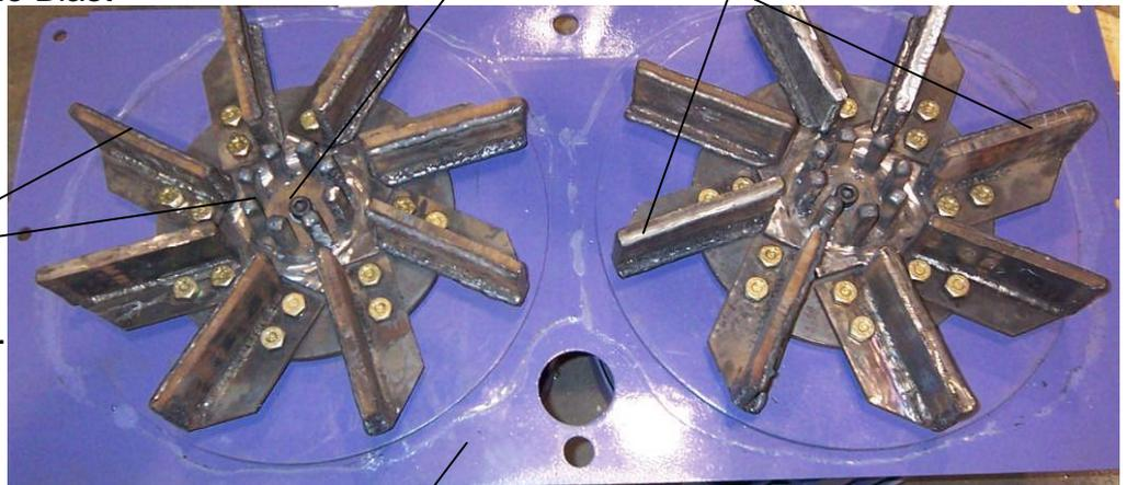
Note: In this photo, the Motor Mounting Plate Assy. has been removed from the Blast Cabinet for clarity in showing the Blades and Impellers. The blades and impeller can be removed without removing the Mounting Plate.
