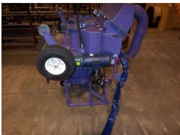
Set the machine back down on the ground and attach the turnbuckles. The turnbuckles assure that the machine is pulled up the wall in a level manner keeping the seal square to the wall. The turnbuckles also keep the machine from tipping as the unit is pulled up or lowered down across weld seams.
