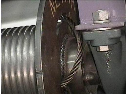
Pull the cable through the drum and out the hole in the opposite side. Clamp the cable in the welded saddle as shown.
