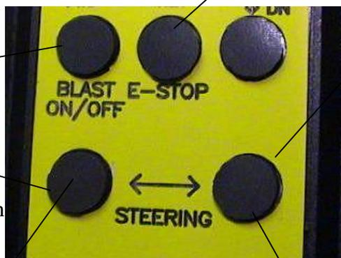
**Steer Right** Bump or tap the button too make slight steering corrections. Hold down longer for turning.
