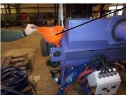
Add 50 lbs of shot in both sides of the machine using the funnel provided. Be sure that the rubber flap is aligned over the adder hole after filling. The flap seals the hole to eliminate vacuum loss. If you lose the funnel provided, they are available at Home Depot.
