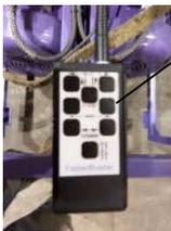
Press the Hoist Up button and lift the machine off the ground and onto the wall. Press the button again to stop the hoist.
