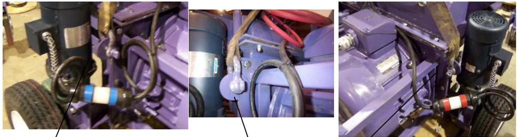
To pick up the machine, place a lifting strap on each side of the machine using a 5/8" shackle in the lifting lugs shown above. The machine is balanced at this point so it will be level.
