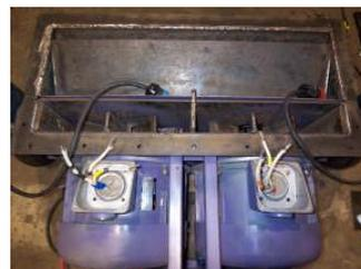
You can now separate the cable harness and the machine panel from the machine.
