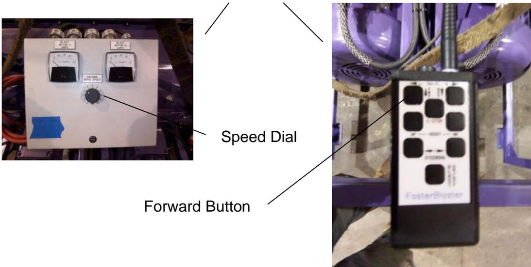
Press the Reverse button on the remote control. The machine will move backwards. Once the machine is moving, you can release the button and the machine will continue moving backward. Press the Reverse button again and the machine will stop.
