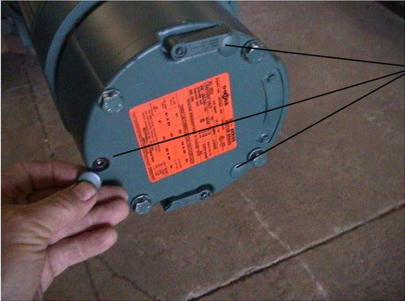
Remove the three plugs on the end of the brake. Tighten each of the three Allen head bolts  $\frac{1}{4}$  turn and try the hoist again. Continue this procedure until the brake works properly.
