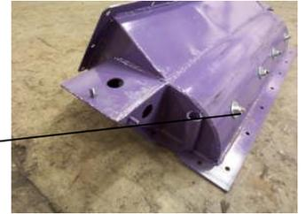
To remove the Top Curved Liners, remove the four nuts and washers on the Blast Hood. Then tap on the studs to loosen the liners.
