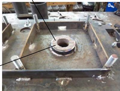
Glue the felt seal in place with silicone
