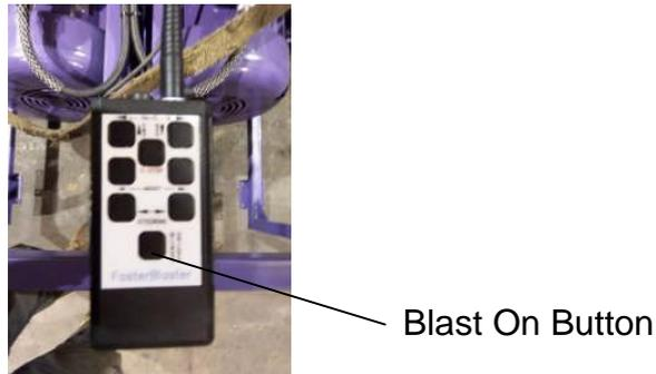
Check the blast motor operation. Press the Blast On button. One blast motor should start. Let up on the button. After a timed delay, the second motor should start.. Check the rotation of the motors. Looking from the back of the machine at the motor fan, the left hand motor should be turning clockwise and the right hand motor should be turning counter clockwise. To stop the blast motors, press the Blast On button again.
