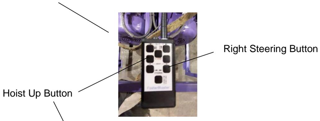
**Step 12** Before loading shot and starting the blast operation, practice running the machine forward, backward and turning at various speeds. You can also shift to full speed momentarily by holding down the Hoist Up button. When you let up on the button, the machine will slow down to the set speed. This is used to turn quickly. Try it.
