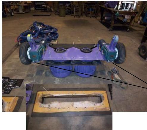
Unbolt the gear box from the support bracket.
