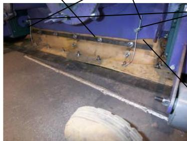
Step 8- Install the four Support Cables from the corner retainer studs to the lock down coupling nuts on the Blast Cabinet, as shown. The cables should be slack enough to allow the seal to float, but tight enough to support the seal assembly when the machine is lifted off the ground.
