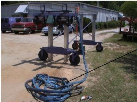
Unroll the power cable so it is free to uncoil as the fixture is lifted to the tank roof.
