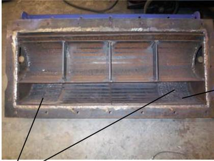
Remove the Top Curved Liners and fill any wear areas with hard face weld. If the wear is too great, replace the liners.
