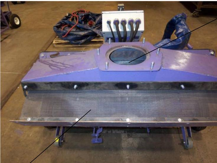
To inspect the screen, remove the exhaust elbow and view the condition of the screen through the round opening.
