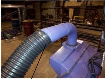
**Caution-** Connect 20' of **High Temp Exhaust Hose** to the machine exhaust elbow and secure with a hose clamp.
