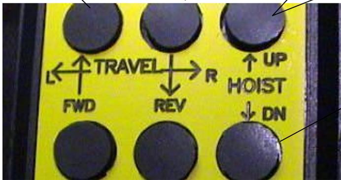
Press until the machine starts moving down the wall then release and the machine will continue moving until you press the button again to stop.
