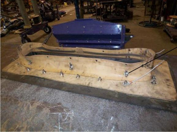
Step 6- Wrap the Vertical Seal around the assembly and attach it over the threaded studs of the Manganese Protector Bars. Install flat washers and lock nuts on the studs as shown.
