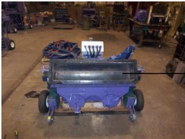
Remove the hood by removing all the bolts around the flange.
