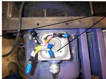
Remove the wire nuts at the blast motor connections and remove the wire cable from the motor connection boxes.
