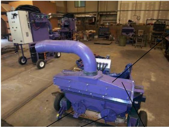
To inspect the blades and liners, unbolt and remove the Blast Hood. With the Blast Hood removed, you can see and inspect the Blades, the Impellers, the Blast Wheel Hub, the End Liners and the Center Liner.
