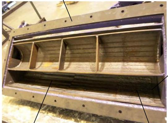
Inspect the Top Curved liners in the Blast Hood
