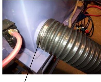
Connect the other end of the exhaust hose to the dust collector. Leave the clamp loose, for now; the hose will have to be adjusted to remove twists and loops after the fan is started.
