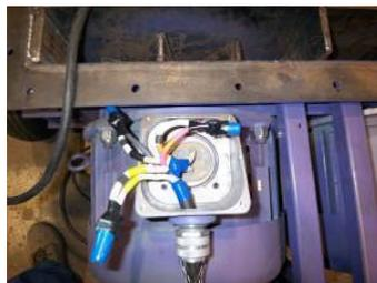
Install the blast motor cables. **Caution-** make sure that the color code on the cables are matched (one is coded with red tape and the other is coded with blue tape). Next, connect the power wires with the wire nuts. All cables are color coded. Add electrical tape around the wire nuts so they can't vibrate loose.
