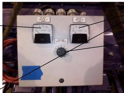
Since the amp meters cannot be seen when the machine is high on the wall, amp meters are also located on the main panel.
