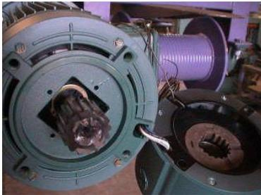
6. Try rotating the brake disc. Blow out any rust or sand lodged between the disc and the clamping plates. Work the disc back and forth until it turns freely. If the disc is still tight, the unit will have to be disassembled for further cleaning. Call RBW before attempting to disassemble the brake.
