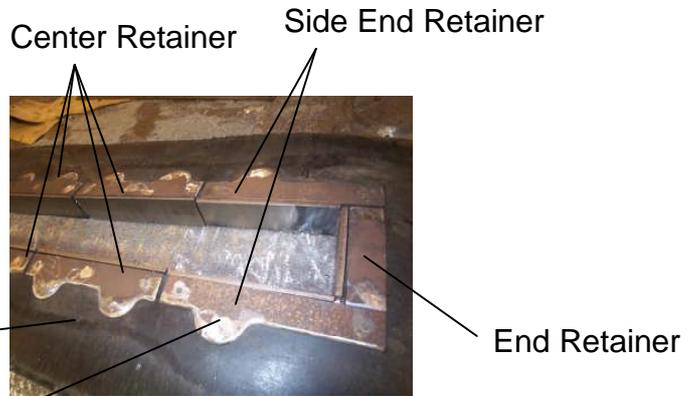
Tapered edge on Main Seal Main Seal
