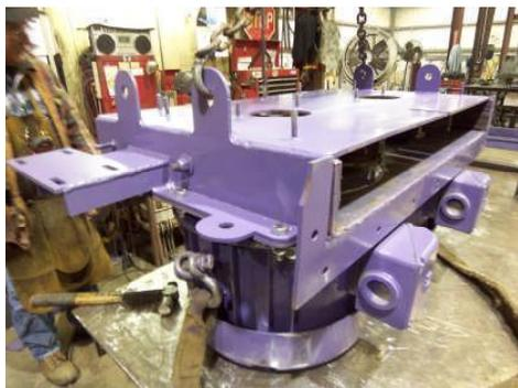
Bolt the the blast cabinet onto the motor mounting plate.
