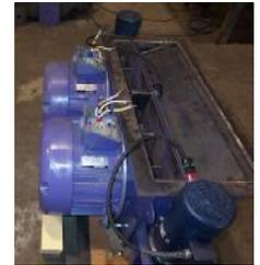
Tip the machine up on the motors, as shown, and remove the two drive tire assemblies and the main seal assembly.
