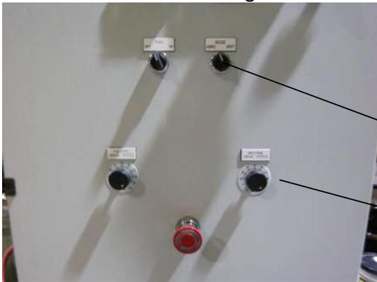
Switch the Mode Selector Switch to Vertical.
