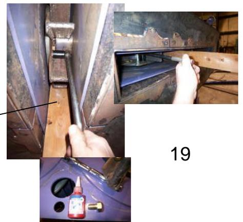
Remove the two end liners by removing the nut on the end wall of the Blast Cabinet. Tap the end of the threaded stud to loosen the liner.
