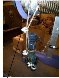
**Caution-**Cable clamp saddles must be placed on the lifting segment of the cable as shown. **“Never Saddle a Dead Horse”.**
