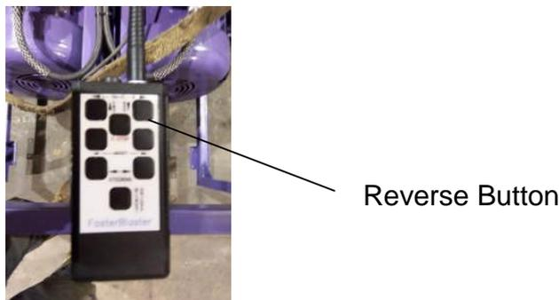
The machine must be moving to turn. Start the machine moving then press the Left Steering Button on the remote control. The machine will turn to the left. Let up on the button, the turning will stop and the machine will continue in a straight movement.
