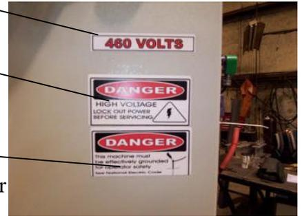
This machine must be effectively grounded for operator safety
