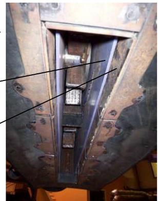
Place the machine on the roof or floor and make sure that the seal is seated tight to the surface and that the support cables are not too tight which would hold the seal up off of the floor. The Cables should have some slack so the seal can float along over wavy surfaces without pulling away from the floor. The cables can be adjusted by loosening the cable locking bolt.
