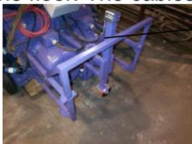
Adjust the level of the machine by cranking the swivel wheel up or down. The blast cabinet should be perpendicular with the floor.
