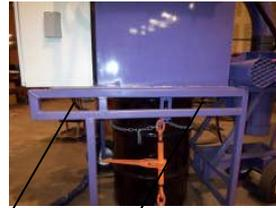
The dust collector can be picked up by a fork lift. Place forks within the frame slots as shown.
