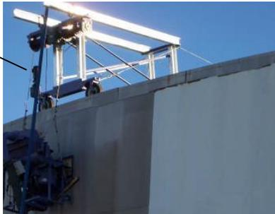
Start the machine moving back down the wall by pushing the Hoist Down Button. After the machine is moving, let up on the switch- the machine will continue to move down the wall until you push the button again.
