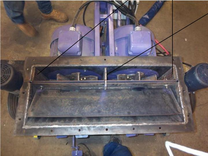
The Center Liner must be removed by driving it up from the bottom side of the blast cabinet with a hammer. Fill any wear areas with hard face welding rod and reinstall by driving it down from the top side of the Blast Cabinet. Drive it down into the notched cutout in the cabinet and the pocket in the Hopper. Be sure to center the bottom of the liner equal distant from the two Blast Wheels. Tap the liner bottom end to the right or left to center it between the two sets of blades.
