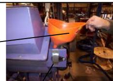
Tape the horizontal flap down to prevent leakage when filling.
