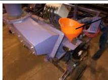
Use a funnel to add shot. Be sure that the rubber flap is aligned over the adder hole after filling. The flap seals the hole to eliminate vacuum loss. If you lose the funnel provided, they are available at Home Depot.
